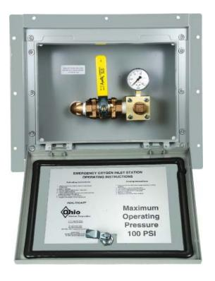
Located inside the emergency oxygen inlet box shall be a 1" (25.4mm) brass ball valve, which can be opened or closed to allow the flow of oxygen. Also included is a 0-100 psi pressure gauge.
