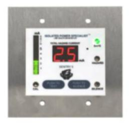
Model SRM-2 wall mounted remote with Red, Green and Yellow LED lamps with a sonalert audible alarm, silence and test switch. Digital meter and LED bar graph all mounted on a pre-polished stainless steel two gang flush plate.
