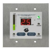
Model SR-1 wall mounted remote with Red, Green and Yellow LED lamps with a sonalert audible alarm and silence switch, mounted on a pre-polished stainless steel one gang flush plate. (Specifications for the <u>SR-1</u>)
